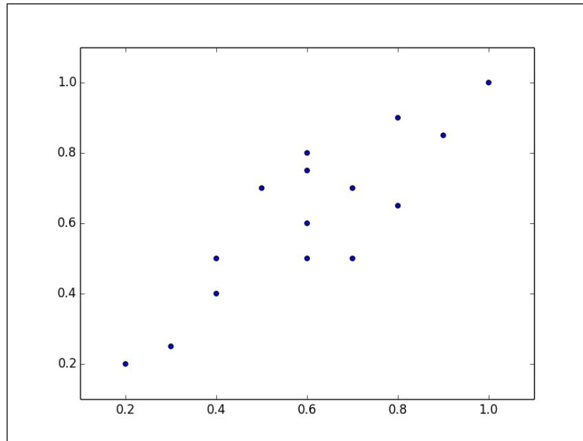
The instances approximately form a long, thin ellipse stretching from the origin to the top right of the plot. To reduce the dimensions of this data set, we must project the points onto a line. The following are two lines that the data could be projected onto. Along which line do the instances vary the most?
