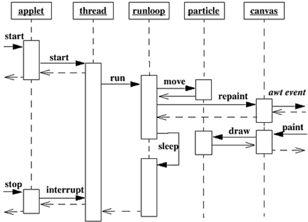
The above interaction diagram shows the main message sequences during execution of the applet. In addition to the threads explicitly created, this applet interacts with the AWT event thread, described in more detail in [§ 4.1.4](#). The producer-consumer relationship extending from the omitted right hand side of the interaction diagram takes the approximate form:
